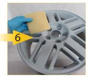
Action: To sand and key awkward areas. **Use:** Mirka Goldflex Soft P500, or Mirka Grey Mirlon Hand Pad. Inspect prior to top coat application.
