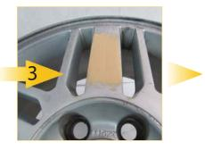
Action: Apply filler to damaged area.
