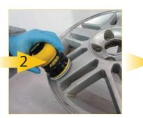
Action: Sand out defects as required. Use: Mirka 77mm Sander with P120 Disc.
