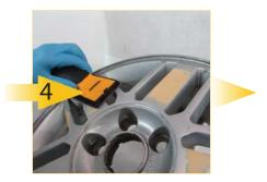
Action: Sand filler area. **Use:** Mirka Abranet P120 followed by P180 Strip. Inspect repair and apply suitable primer.
