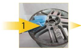
Pre-clean surface to identify damage prior to sanding.
