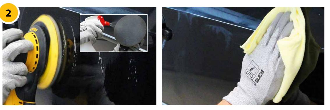
USE: Golden Finish Disc-2. Damp sanding. Spray water on both disc and surface. Sand over surface 3–4 times to achieve a uniform scratch pattern.
