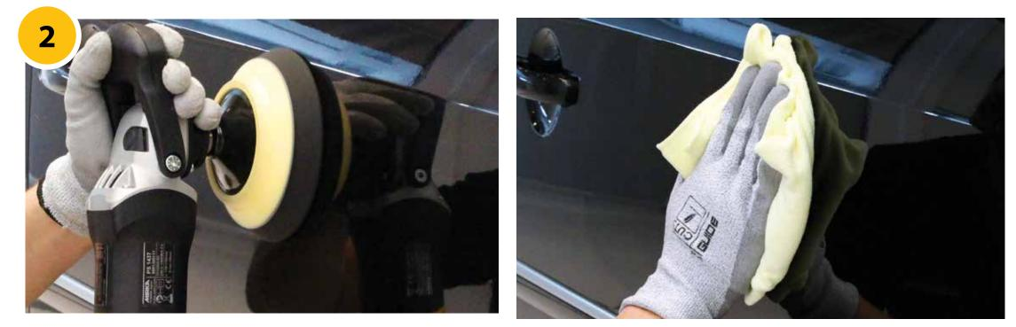
**USE:** Polarshine 5 in combination with Golden Finish Pad-2. Polish until most of compound residue is removed. Keep pad flat against surface. Final wiping with a clean Mirka yellow micro fiber cleaning cloth.
