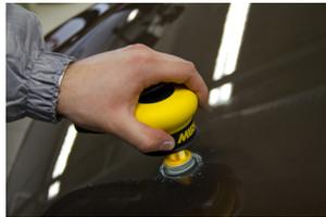
Sand the defect for 2–5 seconds with Polarstar® SR5 using Mirka® ROS150NV machine.
