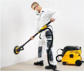
Combine Mirka® LEROS with Mirka's dust-free net abrasives and suitable dust extraction system to create a cleaner and healthier working environment.
